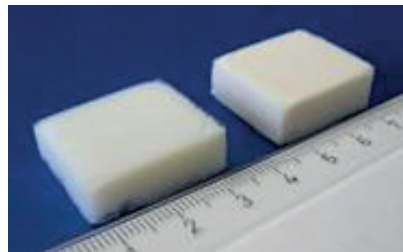
SiO 2 Aerogel with modified MicroFibrillated Cellulose (MFC) fibers, EMPA
