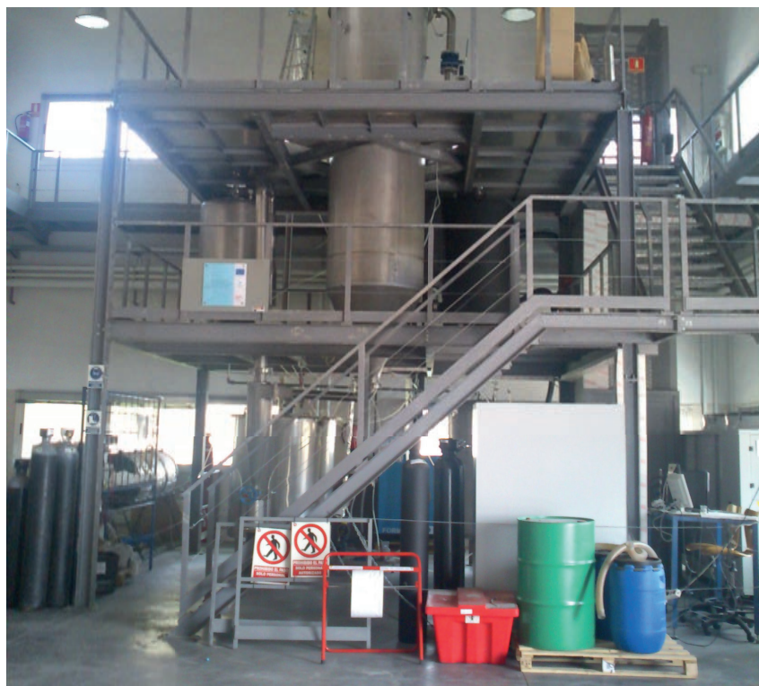
Production plant of NANOPCM additive developed during the project
