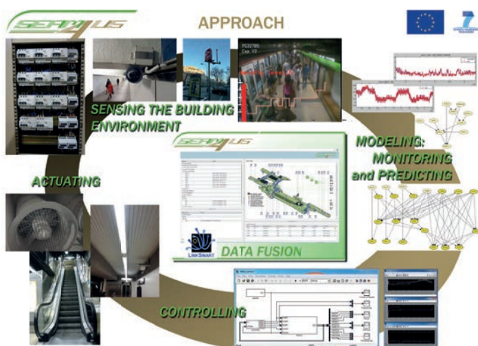
The SEAM4US approach: from the data acquisition using the monitoring network to the implementation of the optimal policies through the models and the controllers
